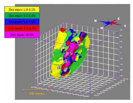
FIGURE 14.18 GRADE SHELLS OF LMZ (104) - HANGING WALL VIEW
