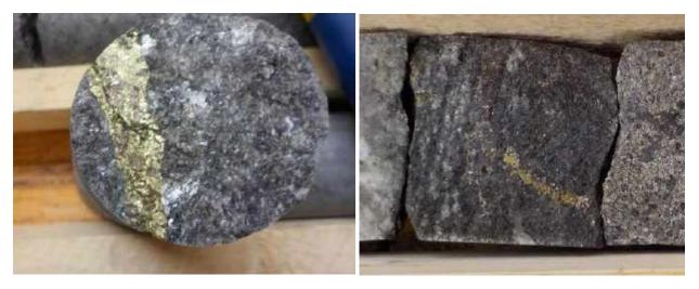
FIGURE 14.7 CROSS CUTTING NATURE OF CHALCOPYRITE
