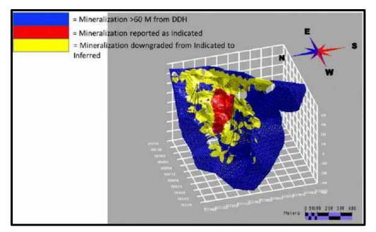
FIGURE 14.10 AREA IN BLUE SHOWS INFERRED BASED ON DISTANCE TO DDH. YELLOW IS AREA DOWN GRADED FROM INDICATED TO INFERRED, RED IN IS AREA CONSIDERED INDICATED
