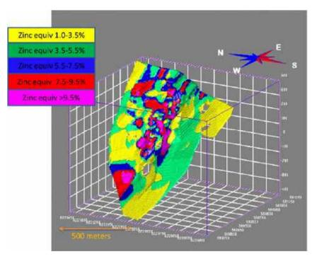
FIGURE 14.17 GRADE SHELLS OF UMZ (105) - HANGING WALL VIEW
