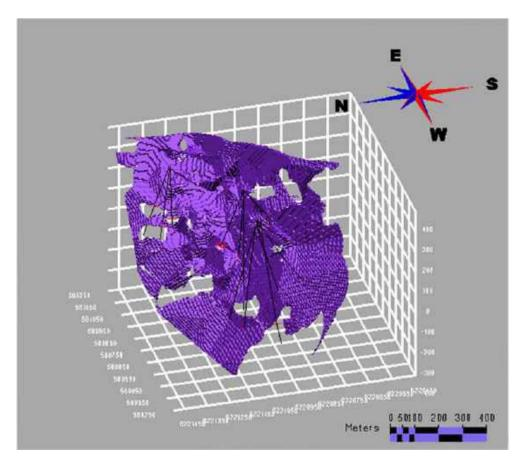
FIGURE 14.14 SHOWING CONTINUITY OF 3.5% ZINC EQUIVALENT GRADE SHELL (PURPLE)
