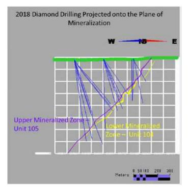
FIGURE 14.2 2018 CROSS-SECTION OF UMZ AND LMZ AS MODELED IN MINESIGHT WITH 2018 DIAMOND DRILLING PROJECTED ONTO PLANE
