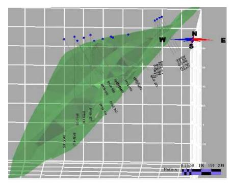
FIGURE 26.5 SECTION LOOKING WEST OF BRABANT MCKENZIE PROPOSED DIAMOND DRILL SITES
