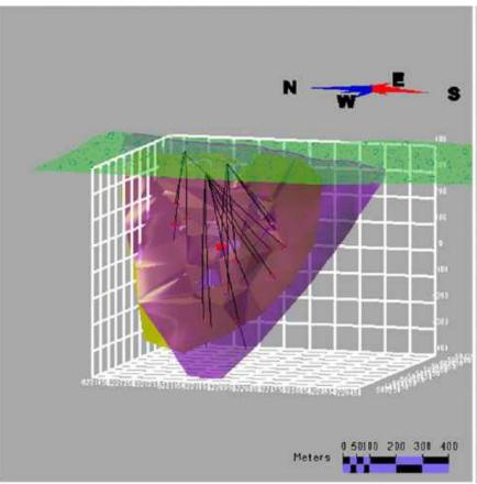
FIGURE 14.1 UMZ AND LMZ AS MODELED IN MINESIGHT SHOWING 2018 DIAMOND DRILLING
