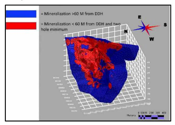
FIGURE 14.9 MINERALIZATION AS DEFINED FROM DISTANCE TO DIAMOND DRILL HOLE
