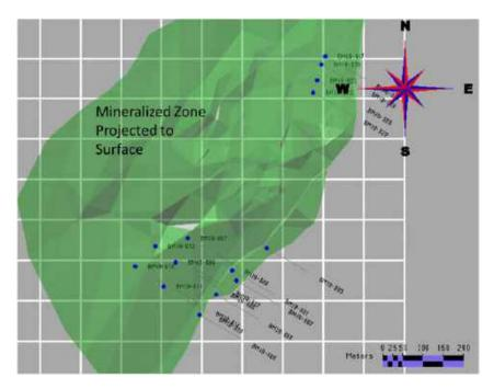
FIGURE 26.6 PLAN VIEW OF BRABANT MCKENZIE - PROPOSED DIAMOND DRILL SITES
