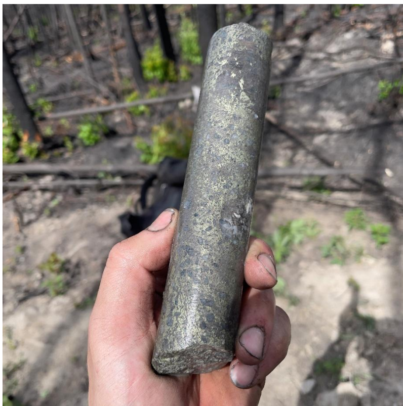
Figure 2: Newly discovered chalcopyrite rich (copper sulphide) mineralization in backpack drill core from the BMK Deposit (Backpack Drillhole NT07221607)
