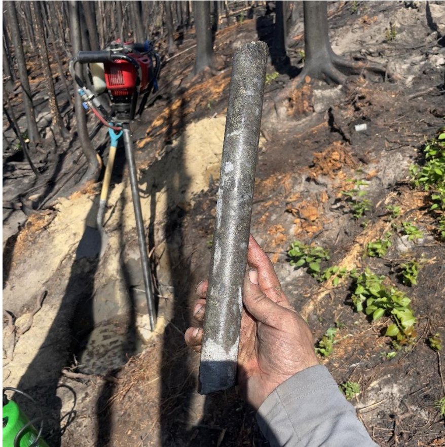
Figure 3: Newly discovered sphalerite rich (zinc sulphide) mineralization in backpack drill core from the BMK Deposit, note the backpack drill in the background (Backpack Drillhole NT07231612)
